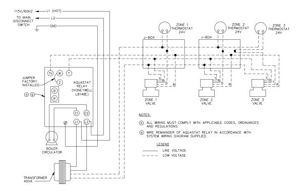
Figure 6.5: Zone Wiring with Zone Valves
